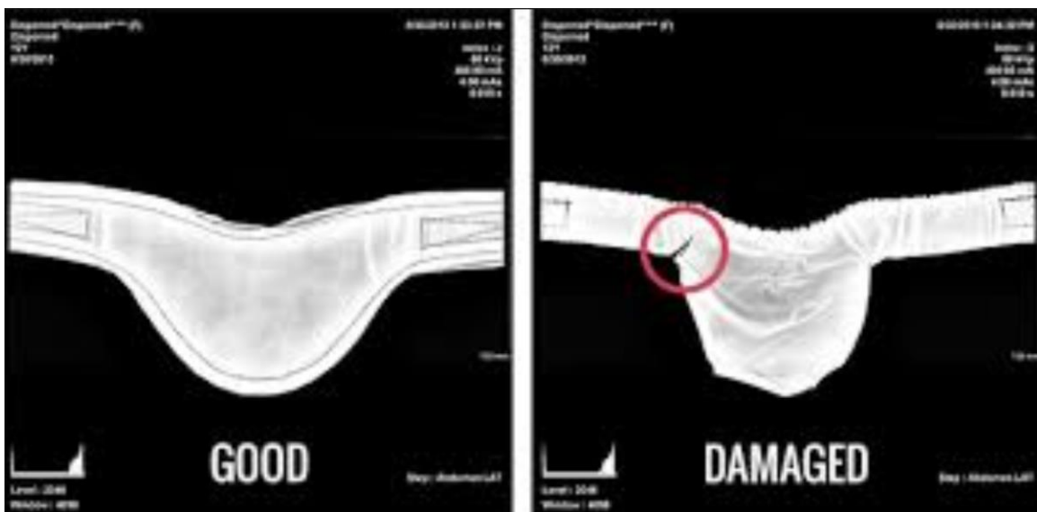
Figure 3 Good and Damaged Lead Apparel
